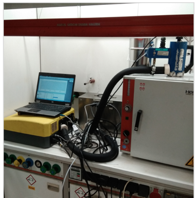
Foto 5: FTIR (Fourier Transform Infrared) Gasanalysator
